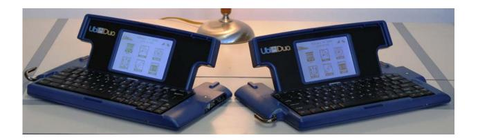
UbiDuo is a portable, wireless, battery-powered, stand-alone communication device that facilitates simultaneous face to face communication by means of two displays and two keyboards.
