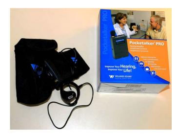
Pocketalker is a portable device that works by amplifying sound picked up through a microphone and sending it straight to ear buds.
