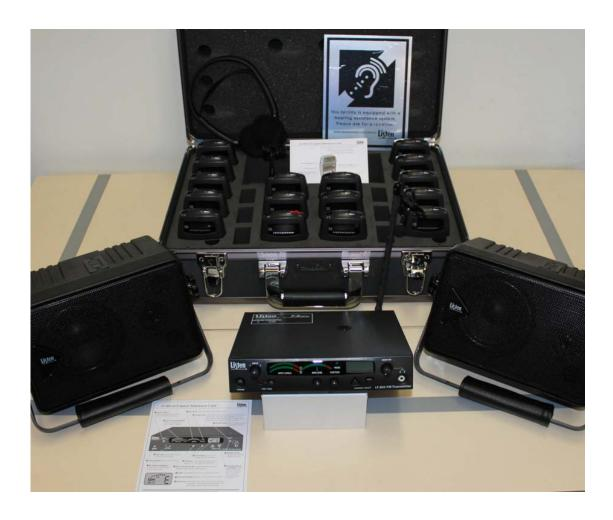
FM Listening system is a portable wireless listening system. In a public setting a speaker may wear a microphone and transmitter that sends his or her voice to a receiver equipped with earphones or a neck loop that works with participants' hearing aids. This device is equipped with 20 receivers and is suitable for large conferences.
